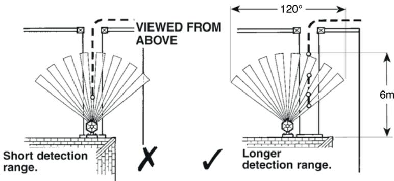
**NOTE:** When the lantern is positioned directly facing a person walking straight towards it, the detection range can be as little as 1.5 metres. We therefore recommend that the lantern be positioned to the side of the entrance.
