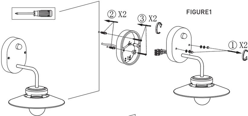
2. Use the backplate as a template and mark positions for fixing holes and cable entry. If fixing it to masonry, drill the fixing holes 25mm deep and insert masonry plugs so they are flush with the surface (FIGURE 2).
